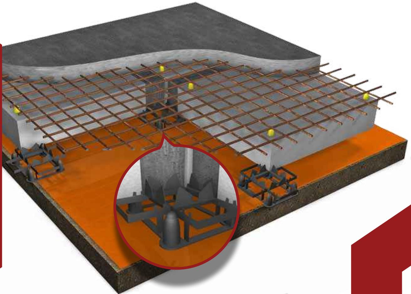
This unique and simple design ensures the Diamond Pods are secure when sites are exposed to high wind areas, and maintains the correct spacing between the pods during the concrete pour.
